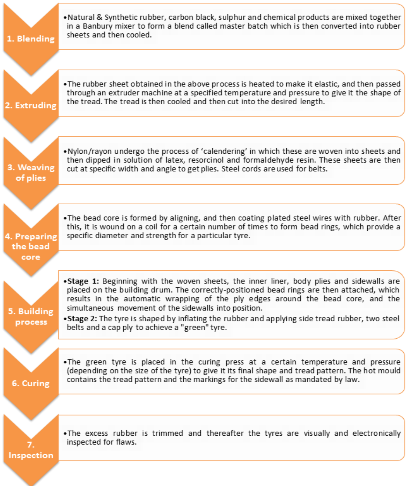
Chart 1: Tyre manufacturing process
